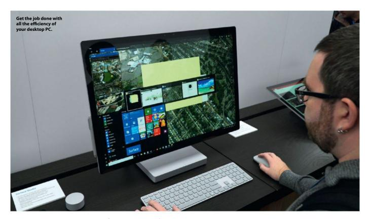
memory and the hard drive - into the tiny base that holds the 'zerogravity hinge'. This hinge absorbs all of the torque required to move the 13-pound display, making it amazingly easy to switch between its standard desktop PC orientation and that of a big drawing surface.
